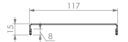
REINFORCING CHANNEL I DETAIL
